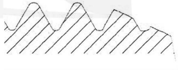
Without R-Processing on Chamfer
